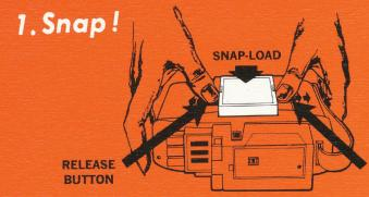
Snap in Snap-Load Magazine. Don't be alarmed at motor hum — Fotron is winding film to first exposure. In approximately 20 seconds, indicator will show 10 "Pictures Remaining" and automatically stop.
